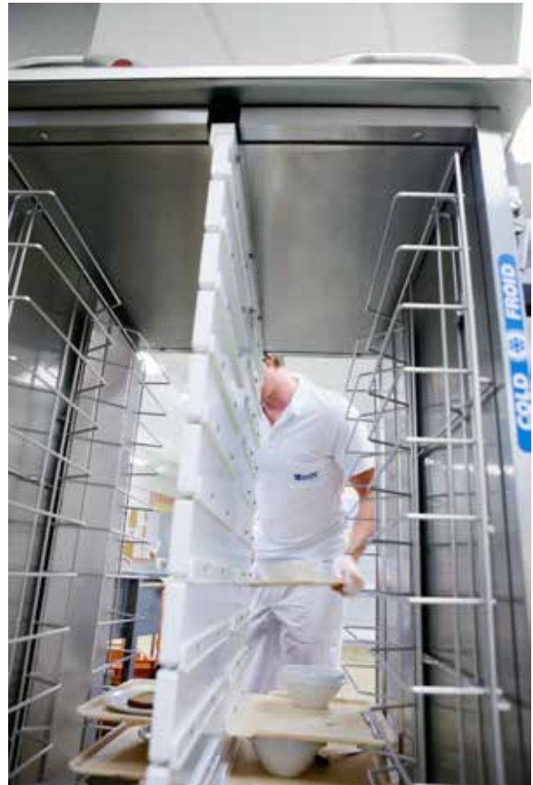
One person can easily handle the machine. As the doors operate automatically, it is easy to load and unload the machine. Just push at button to start the washing. The machine's display shows the progress of the washing cycle.
